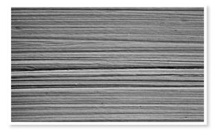
Clearly surfaces on this nature have the propensity to trap dirt and contaminants whilst their roughness hinders proper cleaning as well as an even formation of the passive layer. Equally, it can be seen that orientation of the finish in service will also have an effect with vertical orientation of the 'scratches' being preferred.
