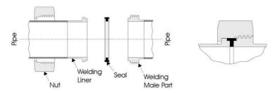
The illustration above shows the assembly of an IDF union with welded parts.
