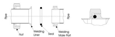
The illustration above shows the assembly of an RJT union with welded parts.
