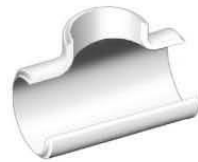
Dimensions (based on ASME/ANSI B16.9) and example weights for equal tees
